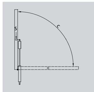
In this position, the point of gravity S is close to or directly on the pivot point. A weak spring force is required. Both strokes are fully extended.
