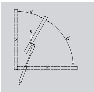
In this position, the point of gravity S moves closer to the pivot point. A weaker spring force is required. Stroke 1 is extended in this position. The spring part 2 with the weaker force now becomes effective.
