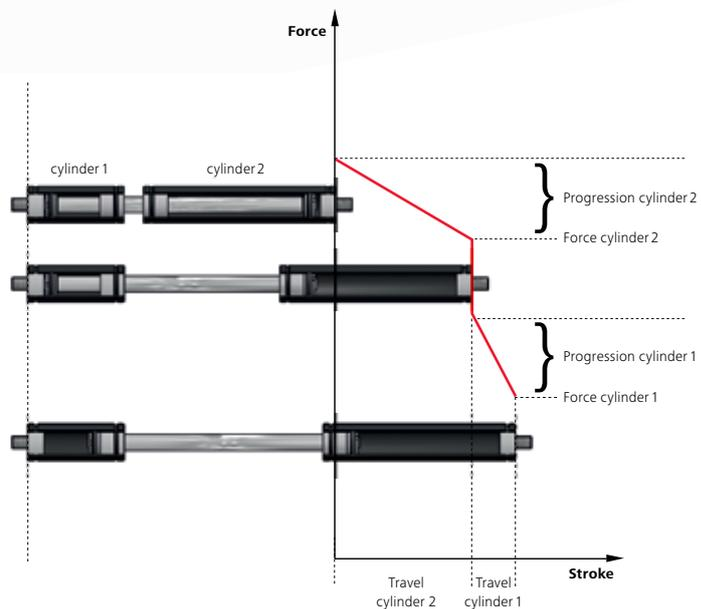
Hahn Gasfedern has developed special double-stroke springs for heavy flaps with a large opening angle, which are characterized by a low starting and a high ultimate force. These springs have two pressure cylinders that can be filled differently and thus are able to cover two force ranges. The compression of the piston rod generates a bent characteristic curve, which can be better adjusted to the force progression of the flap.
